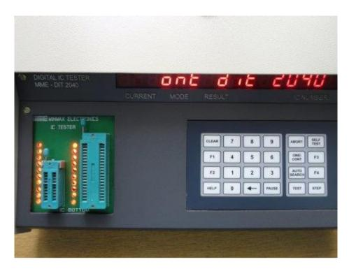
It is microprocessor based digital IC tester from Minmax Electronics .Its functionality tests a variety of digital ICs including Microprocessor, Peripheral IC's, EPROMs, RAMs etc., apart from the standard 74 & 54 series of TTL ICs and 40 & 45 series of CMOS ICs.
