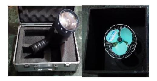
This Xenon tube based Stroboscope is used for the observation of rotating object like still condition. By the help of this RPM, running crack etc. can be measured & observed. In this kit consist of the following items:-
