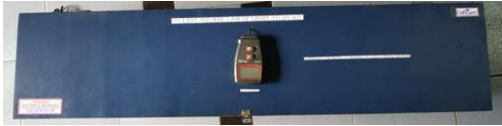
INVERSE SQUARE LAW VERIFICATION EXPERIMENT SETUP
